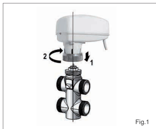
Actuator - valve coupling by means of threaded ring nut
