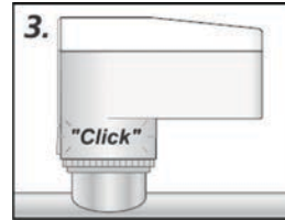
3. Simply latch the actuator to the valve adapter manually by applying vertical pressure; a clicking sound can be heard.
